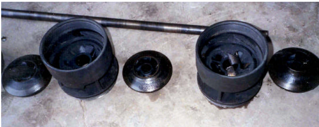
Figure 12. 5th impeller, 5th bowl, 6th impeller, and 6th bowl.
