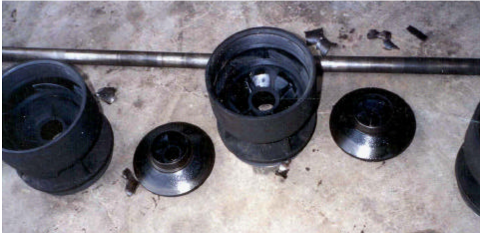
Figure 10. 3rd bowl, 4th impeller, 4th bowl, and 5th impeller.
