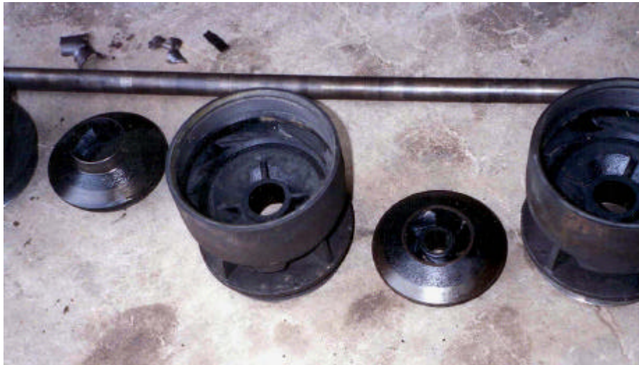
Figure 11. 4th impeller, 4th bowl, 5th impeller, and 5th bowl.
