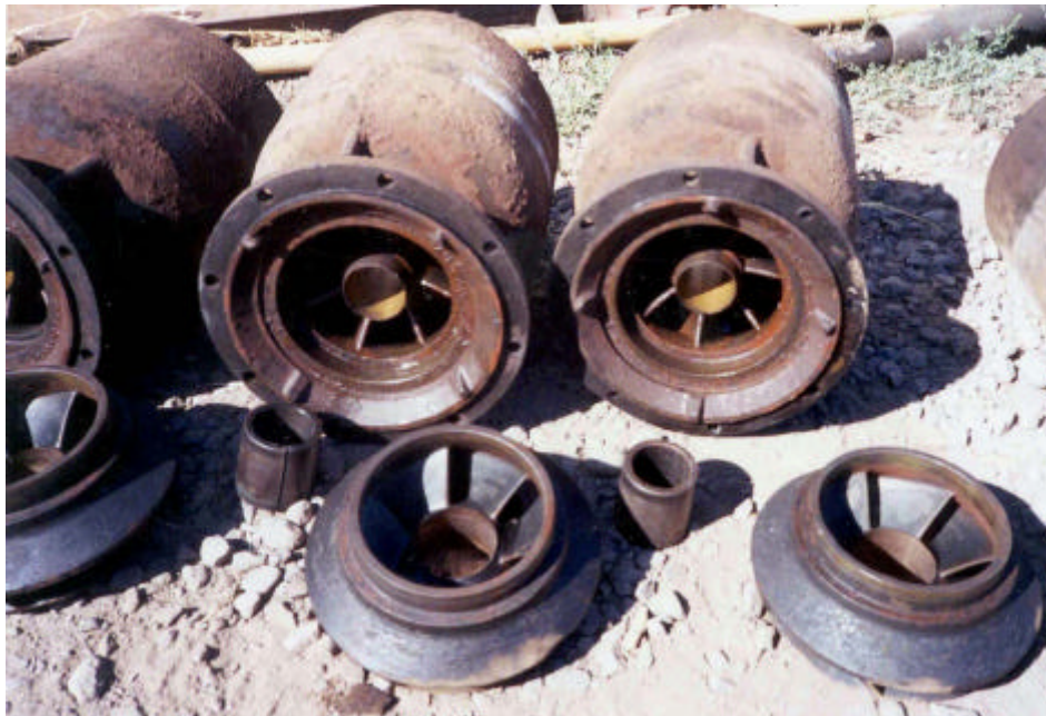
Figure 3. OIT #5 10th and 11th bowls, and impellers
