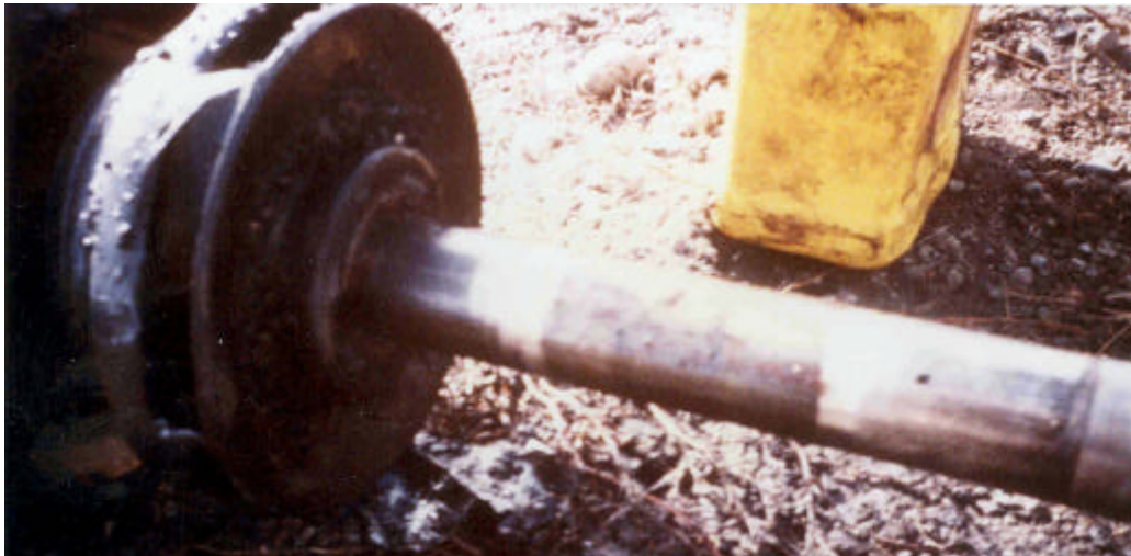
Figure 6. MWMC 1st stage impeller and discolored shaft.
