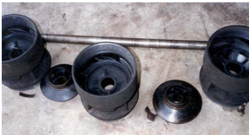
Figure 9. Top bowl, 2nd impeller, 2nd bowl, 3rd impeller, 3rd bowl, and missing bearing remains.
