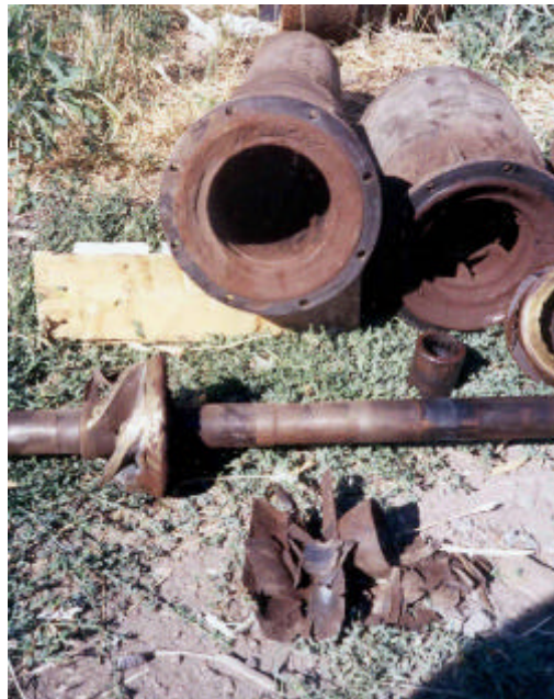
Figure 1. OIT #5 suction case, 1st bowl and impeller.
