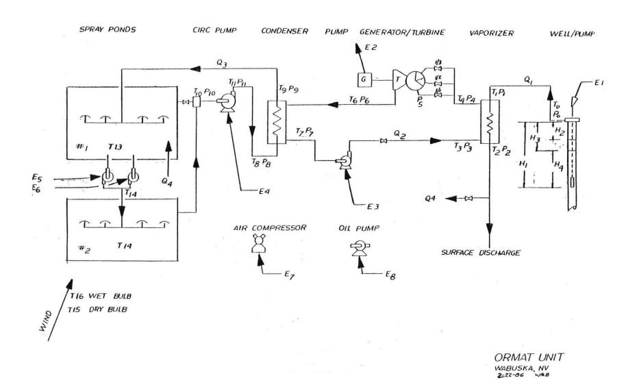
**Figure 1-1** Instrumentation Points
