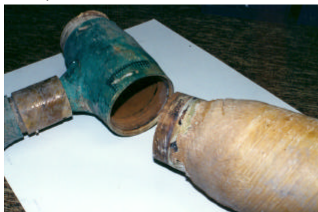
Lock ring portion of joint detached from fiberglass piping.
