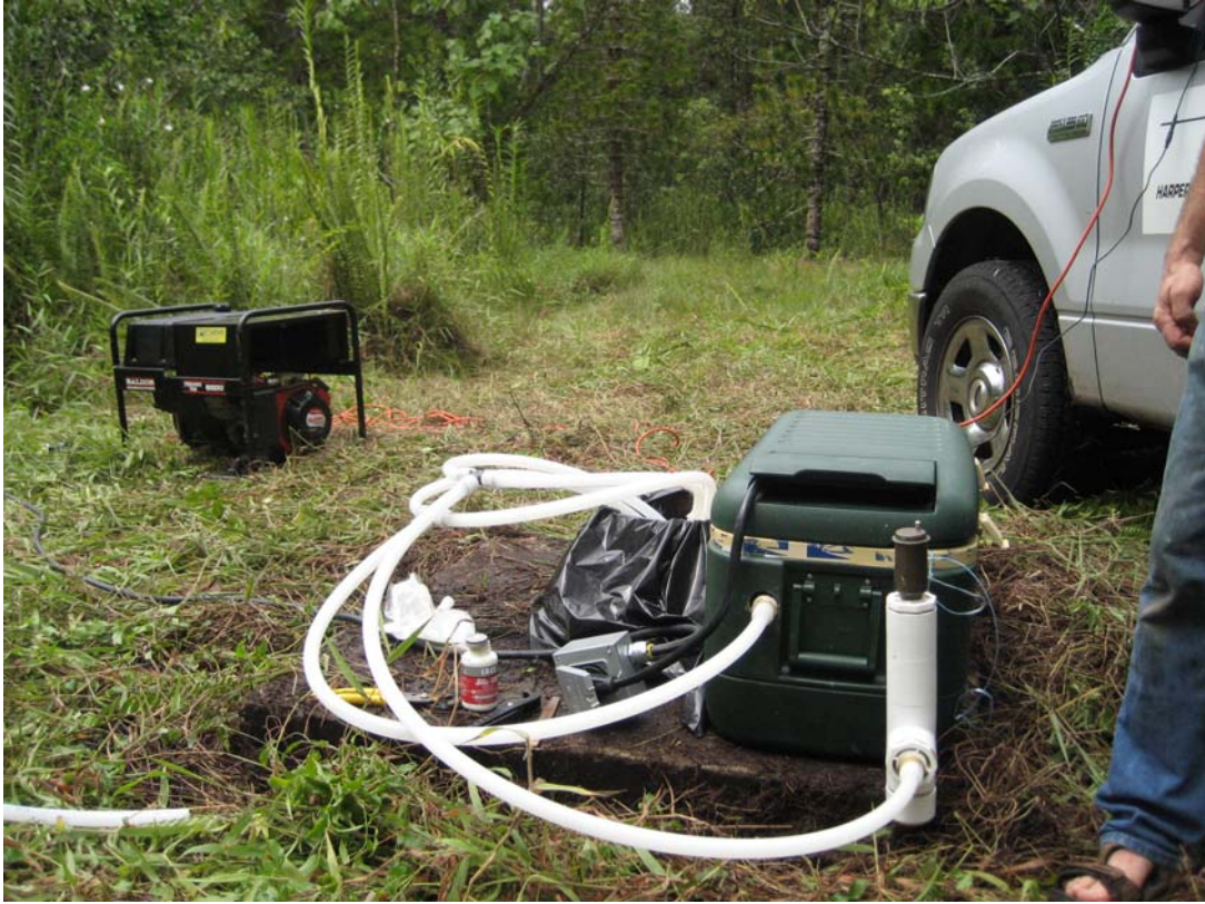
Figure 4. Photograph of the thermal response test setup.
