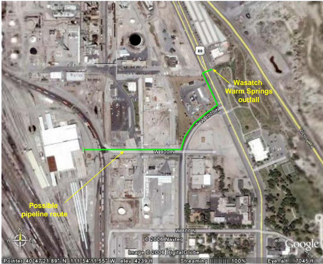
Figure 9. Possible pipeline route to the UTA facility from the Wasatch Warm Springs.
