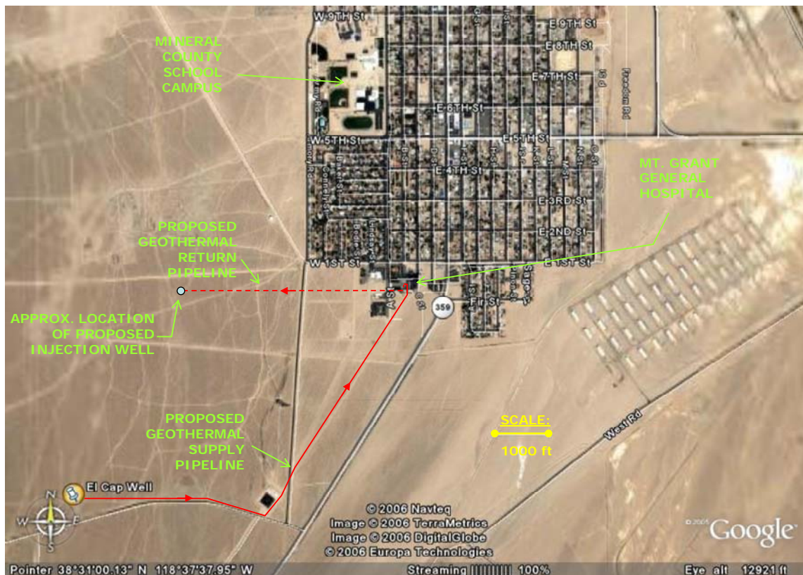
Figure 5. Proposed layout of geothermal supply and disposal pipelines.
