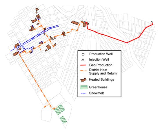
Figure 1. Klamath Falls Geothermal District Heating system location map, 2005
