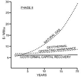
Figure 2. Phase II Unit Energy Cost Comparison (Lineau, 1981)
