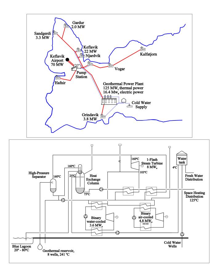
Figure 1. The Sudurnes Regional Heating System layout and flow diagram for Svartsengi Power Plant.
