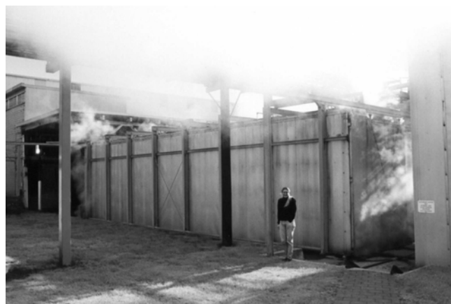
Figure 3. Reconditioning of the dried lumber.
