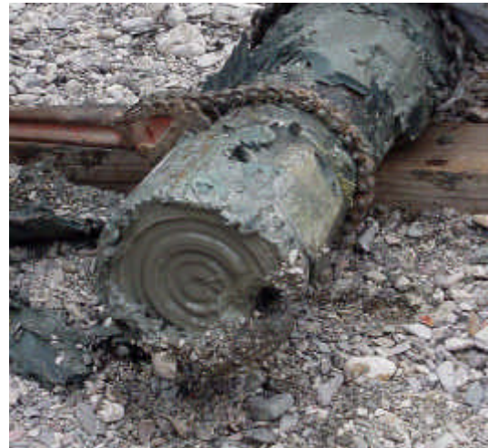
Figure 4. Drilling bit with clay.
