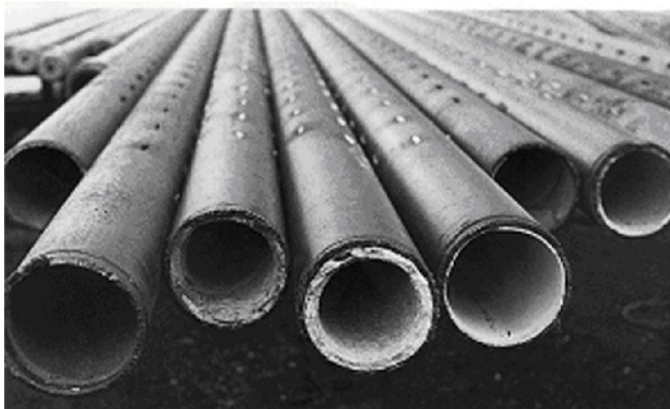
Figure 9. Calcite scaling in Krafla, Iceland well liners.
