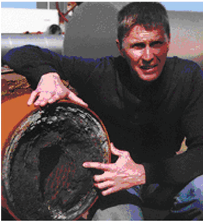
Figure 8. Calcite scaling in surface pipes.
