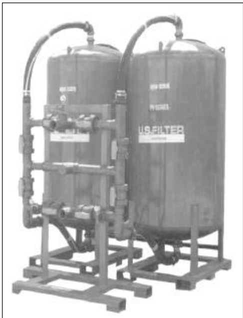
Figure 5. Activated carbon filter.
