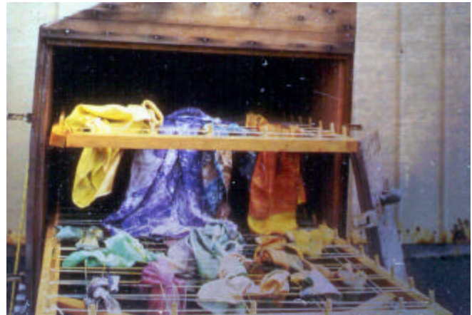
Figure 7. Samples of the hand-dyed silk treated with raw geothermal steam (Camera Hawaii, Inc., 1987).
