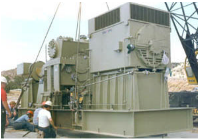
Figure 6. Skid-mounted biphas turbine system operated at Roosevelt Hot Springs (photo from www.douglasenergy.com ).
