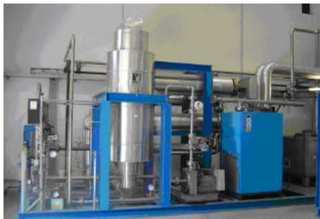
Figure 5. Installation for cleaning and drying CO 2 gas produced from well Blumau 2.
