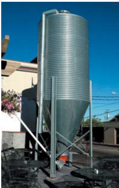
Figure 2. Photograph of the malted barley silo.
