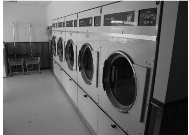
Figure 6: New Retrofitted 55 lb. Dryers
