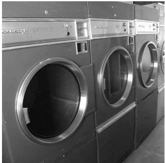
Figure 3: Decommissioned Commercial 30 lb. Gas Dryers
