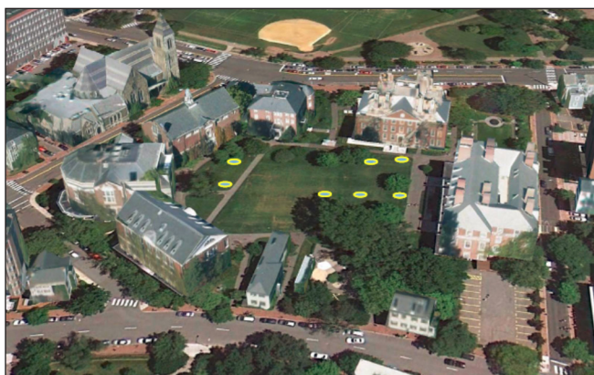
Figure 3. A bird's eye view of Radcliffe Yard showing the five well Byerly System (on the right) and the two well Gym system (on the left.) Haley & Aldrich, Inc.
