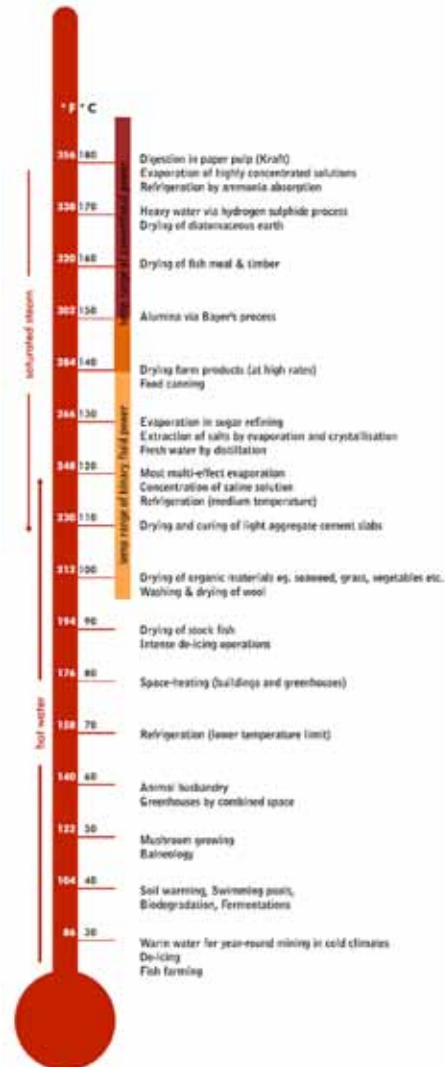
Figure 12. Utilization of geothermal energy at different temperatures (Lindal, 1973).
