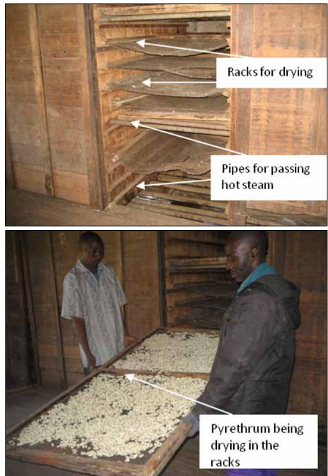
Figure 2. Geothermally heated pyrethrum drier.
