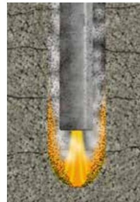
Figure 4: Hydrothermal Spallation (Potter Drilling, 2012).
