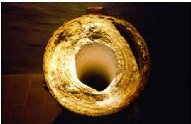
Figure 5. Scaling in geothermal pipeline (Bloomquist, 2006).
