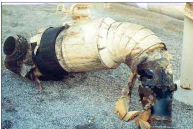
Figure 8. Corroded Steam Vent (Kagel, 2008).
