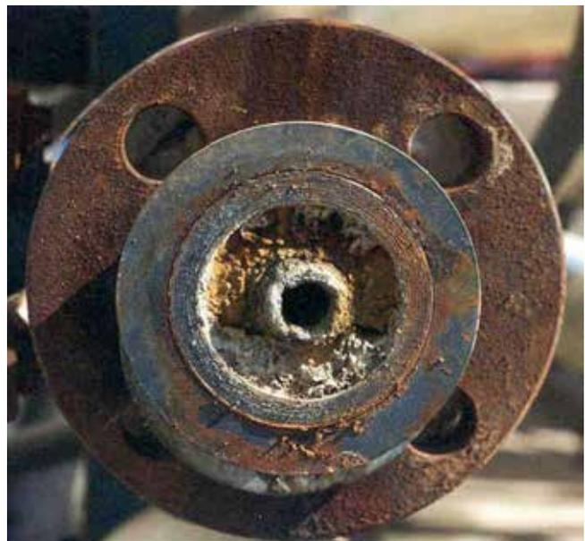
Figure 6. Corrosion of tubes (Kagel, 2008).
