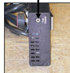
Fan control jacks.
