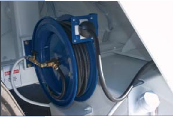
50 foot (15.25 m) long wash-down hose is standard. Longer ones are available.
