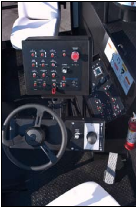
The control panel swivels and can be used from the right-hand or left-hand operator station.
