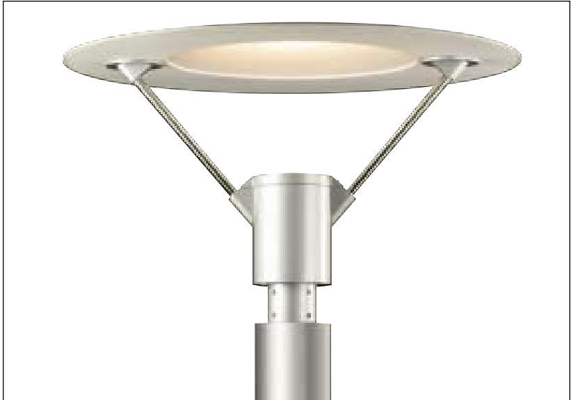
Pole Lighting Manufacturer: Bega Model: 8309, full cut off, 12' height, 5" diameter pole, dark sky Color: BEGA silver
