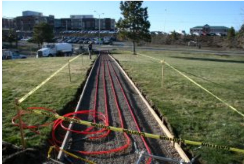
Figure 2. Seismic testing for the deep geothermal well in Spring 2008 (Photo credit: Kristina Maupin).
